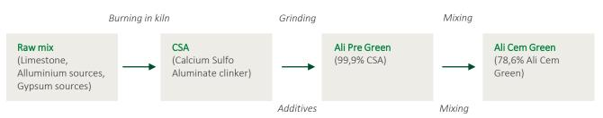
The overall composition of the products under study and the energy input involved are provided below. This shows relative percentages of materials and energy sources used in producing **ALI PRE GREEN** and **ALI CEM GREEN**, without considering loss in mass during combustion.
