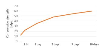
The strength measurement test was carried out on standard mortars according to UNI EN 196-1
